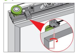
3 Adjust tightness of the wire to and fix it
