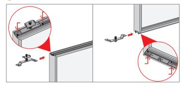
2 Install connection bottom roller to sliding door 2
