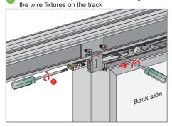
2 If the door panel is not aligned, it can be fine-tuned with this screw
