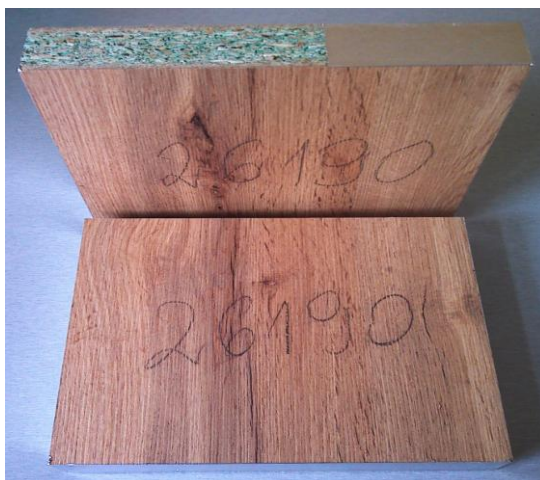
Image 1 Sample for testing according to PN-EN 717-1:2006
