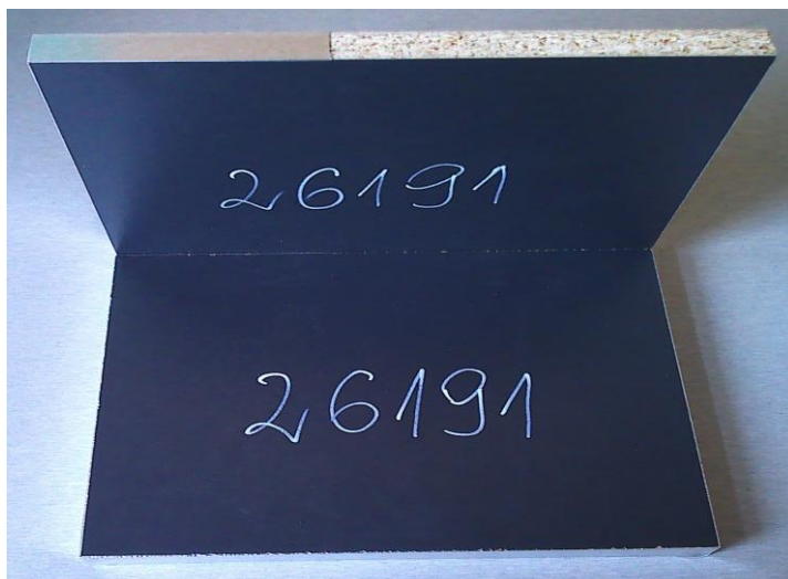
Image 1 Sample for testing according to PN-EN 717-1:2006
