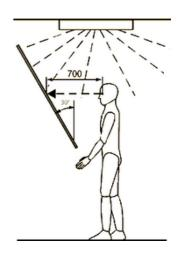
Panel evaluation should take place under a diffuse and fixed light source that illuminates the surface uniformly. This can be sunlight or adequate artificial lighting (between 2000-5000 lux). The approximate distance between the assessed surface and light source should be 1,5m. Surface defects will only be acknowledged if they are larger than 0,8mm<sup>2</sup> and visible from a distance of 0,7m at a viewing angle of approximately 45°.
